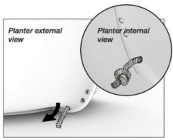
Pull the unknotted end of the rope all the way through the hole until the knot hits the end as shown.
