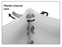
4. When reaching the top hole, thread the rope through the other line of holes on adjacent side. Continue to thread the rope until reaching the bottom of the planter.
