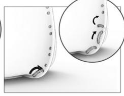
Thread the rope through the next hole above and pull towards the internal of the planter. Thread the rope in alternating in-out pattern as illustrated.
